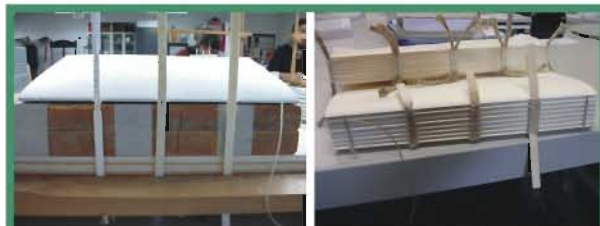
Beginning to sew a text block onto a variety of slotted cords (left) and the finished product (right)
